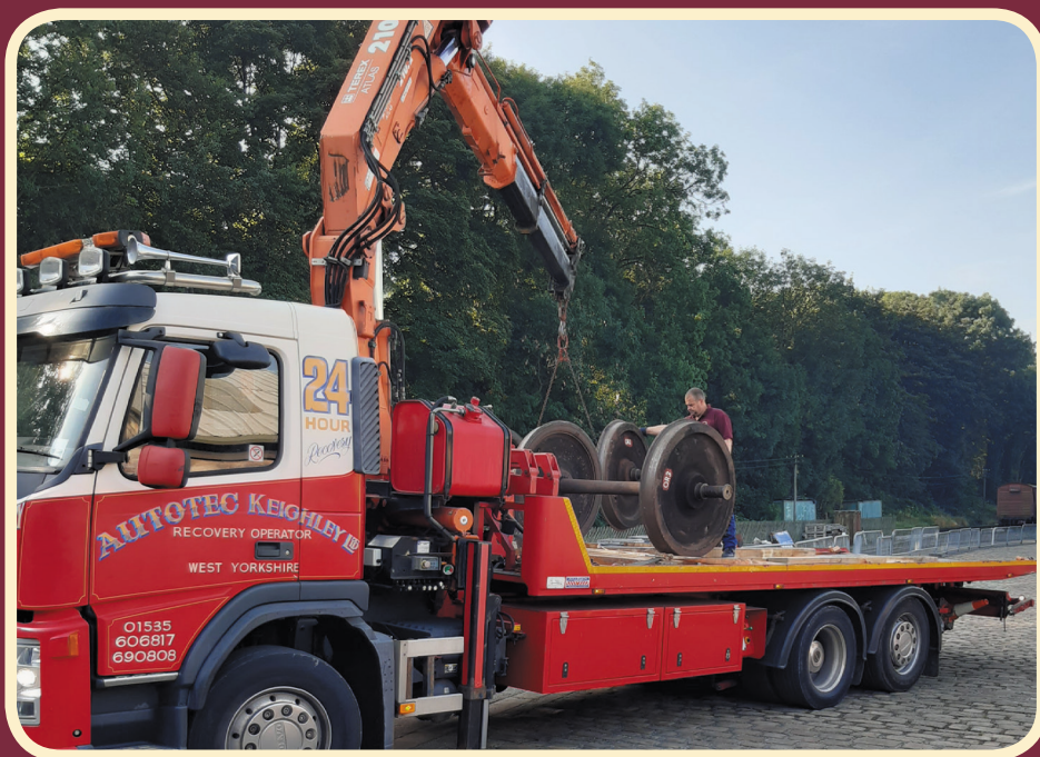
Chris Smith checking the loading of Midland Carriage Wheelsets for Tyre Turning Photo: Bob Sprot
